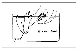
3. While gently pushing down the internal steel ball using stiff wire (0.5 mm diameter), move the plunger through 5 to 10 strokes until it slides smoothly. This will remove dirty oil from the lash adjuster and loosen the plunger.
