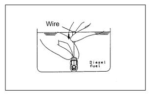
Place the lash adjuster in container C. Then gently push down the internal steel ball using a stiff wire (0.5 mm).
