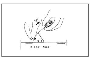
6. Remove the lash adjuster from container B. Then gently push down the steel ball and push the plunger to remove the diesel fuel from its pressure chamber.
