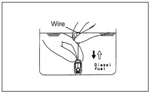
8. Stand the lash adjuster upright with its plunger at the top, then push the plunger downward firmly until it moves through its furthest possible stroke. Return the plunger slowly, then release the steel ball and allow the pressure chamber to fill with diesel fuel.
